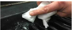
Before any repair, grease, oil and soap must be removed from the area to be repaired. Repair any leakage detected using Marine Flex Silicone.
