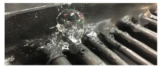
Inspect both sides of the sleeve for signs of leakage by using a leak indicating solution (soap water). Small indicating leaks (bubbles) are acceptable as long as the leak is only from one side of the penetration only.
