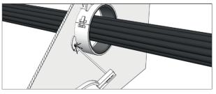
Fasten the graphite collar to the bulkhead or deck by welding. Use FireSeals welding lugs.
