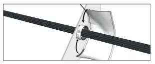
Take the openable wrap, remove the film from the tape and place it on the collar. Secure the wrap with the supplied cabel tie.
