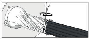
Secure the cable tie over the cables
