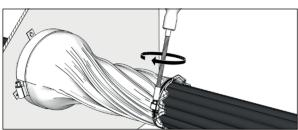
Secure the fireproof wrap with the supplied cable tie. Use a Hex 7mm/Ph2 screwdriver.
