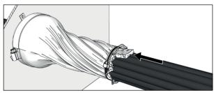
Fill any gaps between cables and/or cable and the wrap with enclosed Marine Blanket. The spare Marine Blanket is placed inside the wrap.
