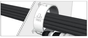
Fasten the graphite collar to the bulkhead or deck with the enclosed self-taping screws.
