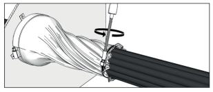
Remove or loose the cable tie holding the cables
