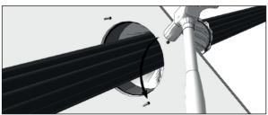
To avoide cut hazard, it is opptional to remove the drillingtip by useing a pliers, hammer or a pipe with an inner diameter of Ø6mm.
